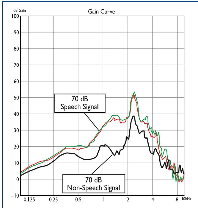
Figure 1. Comparison of speech and non-speech signal in an advanced digital hearing instrument with DNR.
