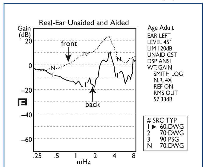
Figure 2. Comparison of a 70 dB signal with the user facing the speaker versus turned 120° to the left.
